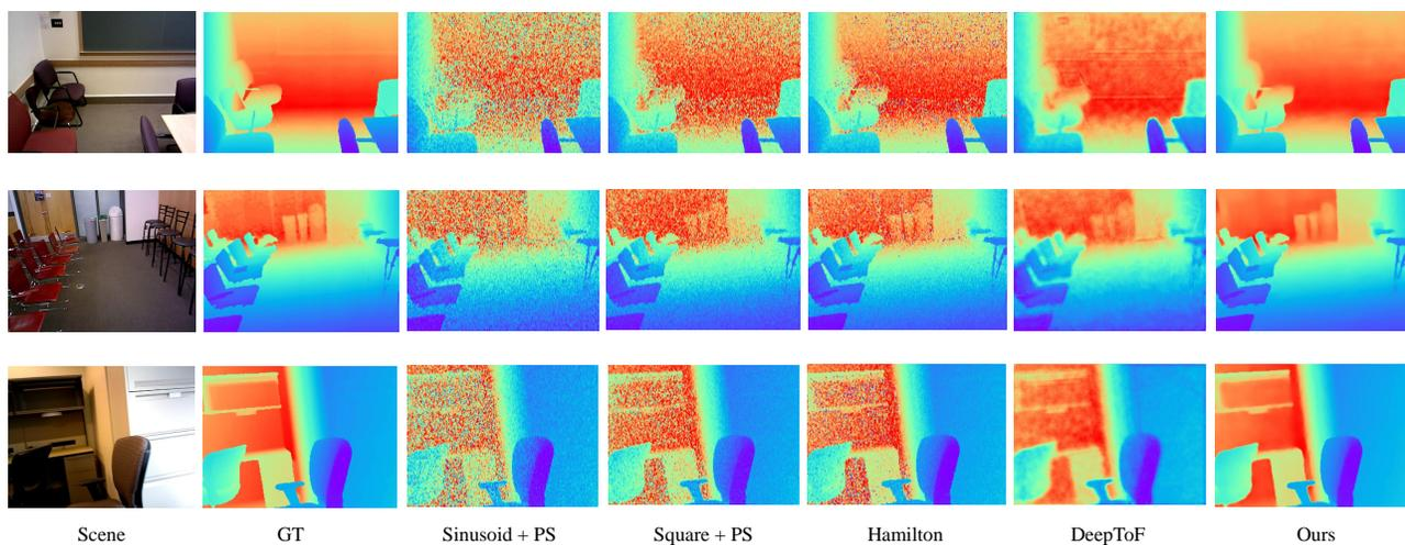
Figure 4. Depth reconstruction results on SUN RGB-D dataset [7] under small noise level, i.e.  $(E, \beta) = (20000, 6000)$ .
