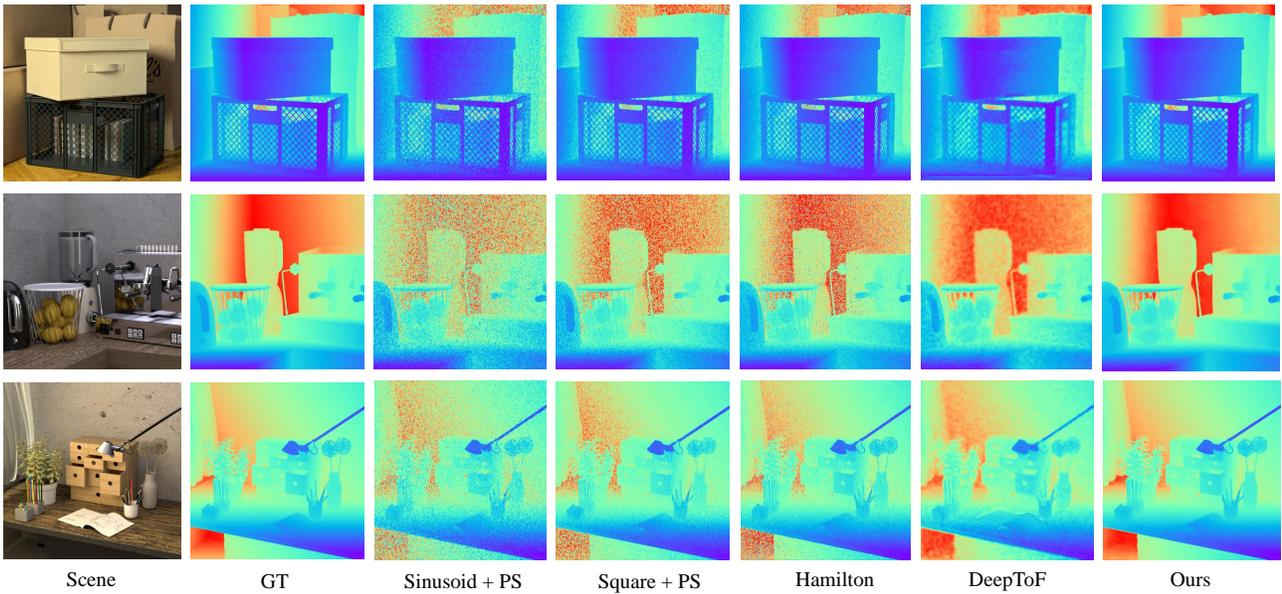
Figure 2. Depth reconstruction results on 4D Light Field Dataset [5] under middle noise level, i.e.  $(E, \beta) = (14000, 6000)$ .
