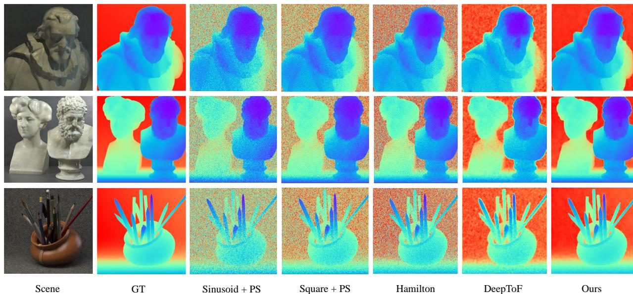
Figure 3. Depth reconstruction results on 4D Light Field Dataset [5] under large noise level, i.e.  $(E, \beta) = (10000, 6000)$ .
