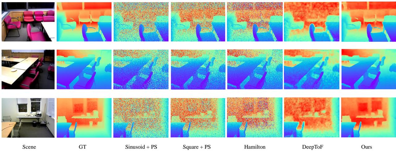
Figure 6. Depth reconstruction results on SUN RGB-D dataset [7] under large noise level, i.e.  $(E, \beta) = (10000, 6000)$ .
